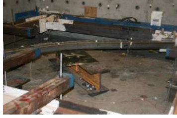
(b) Out-of-plane buckling of IPB brace system[7]
